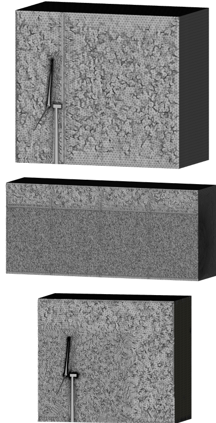
Fig. 28: Meshes used in the MDM wind-turbine aerodynamics and FSI simulations. Top-to-bottom: Turbine 1, Box, Turbine 2.
