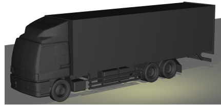
Fig. 15: Truck model. Length: 12.14 m, width: 2.41 m, height: 3.77 m.
