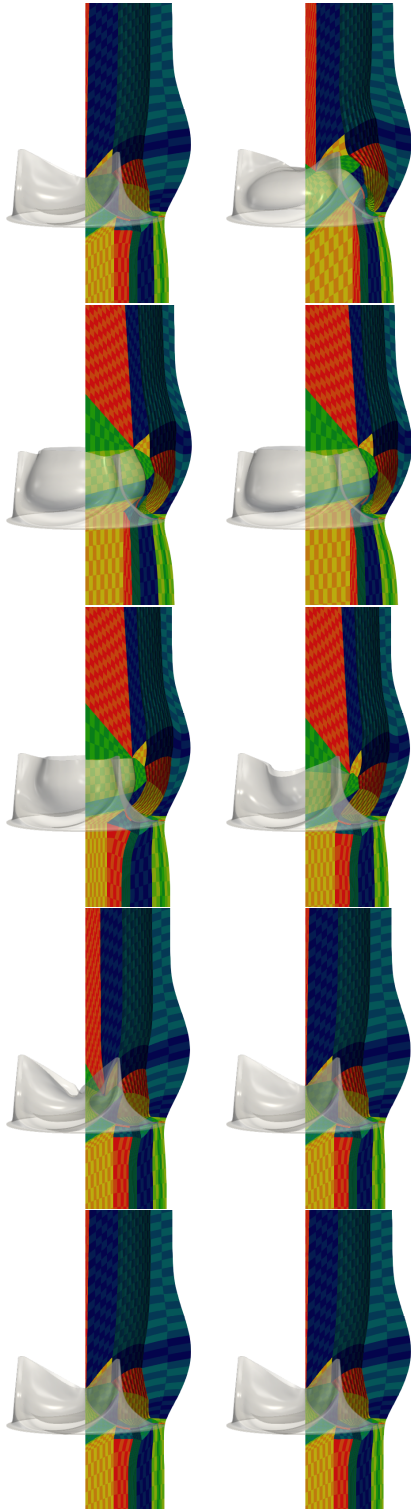
Fig. 10: Flow analysis of a BHV. Cross-section of the mesh at t = 0.175, 0.275, 0.315, 0.495, 0.585, 0.590, 0.595, 0.605, 0.635, 0.785 s. The colors are for differentiating between the NURBS patches. The checkerboard pattern is for differentiating between the elements.
