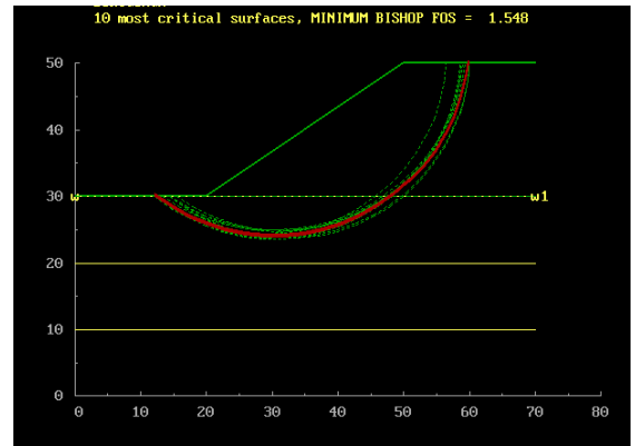
Fig. 8: Display of the 10 most critical surfaces & the minimum factor of safety for Borehole 3 (undisturbed soil).
