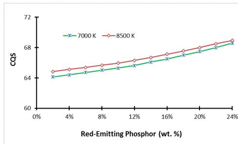
**Fig. 6:** CRI properties of WLEDs with various  $\alpha\text{-SrO}\cdot 3\text{B}_2\text{O}_3\text{:Sm}^{2+}$  concentrations.
