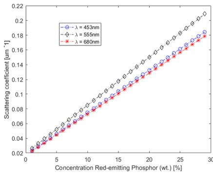
**Fig. 2:** Scattering coefficients of  $\alpha\text{-SrO}\cdot 3\text{B}_2\text{O}_3\text{:Sm}^{2+}$  versus concentration red phosphor (%)
