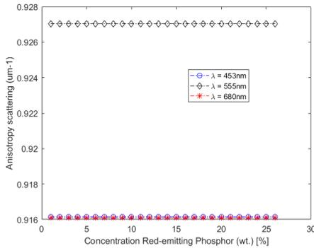
**Fig. 3:** Anisotropy scattering values of  $\alpha\text{-SrO}\cdot 3\text{B}_2\text{O}_3\text{:Sm}^{2+}$  versus concentration red phosphor (%)
