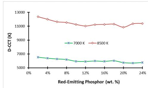
**Fig. 8:** D-CCT of WLEDs with various  $\alpha\text{-SrO}\cdot 3\text{B}_2\text{O}_3\text{:Sm}^{2+}$  concentration.
