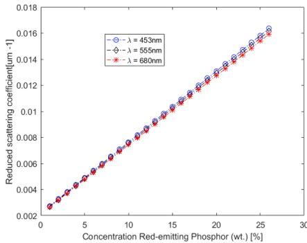
**Fig. 4:** Reduced scattering coefficients of  $\alpha\text{-SrO}\cdot 3\text{B}_2\text{O}_3\text{:Sm}^{2+}$  versus concentration red phosphor (%)
